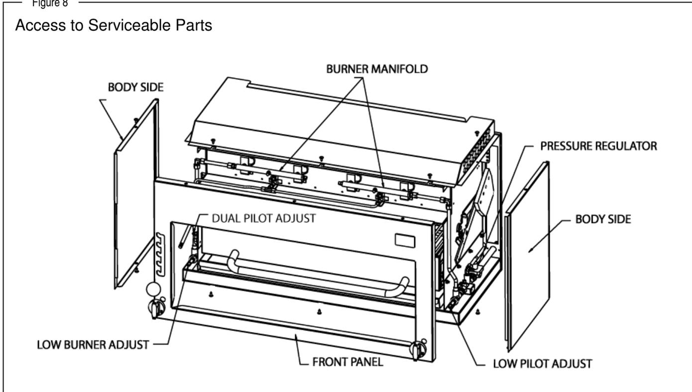
If necessary (or convenient), wall-mounted and flue-riser-mounted models can be un-mounted for servicing or repairs. Use two people since the broiler weighs about 175 pounds (77 kilograms). Refer to the installation procedure in the previous section of this manual for guidance.
