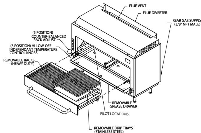
**Keep the bottom drip pan in place when broiling. Without it in place, excessive air is pulled past the burners, reducing temperature and cooking efficiency.**
